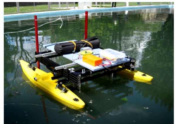
Fig. 2. ASV with crane for multiparameter probe.
